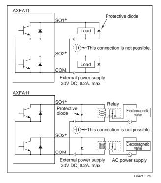
Figure 4.4.13 Status Output Connection
